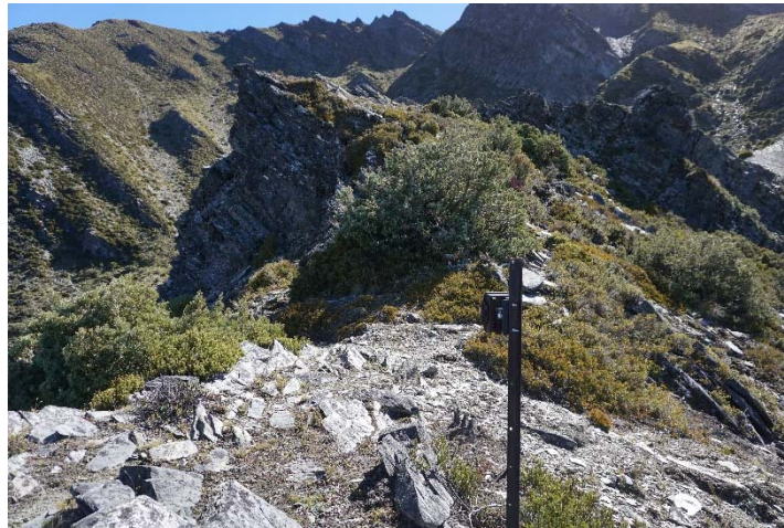
Figure 2. A pole-mounted trail camera located to photograph ungulates on a game trail along a spur above the bush edge, deployed in Timaru Creek, Otago, March–September 2018.
