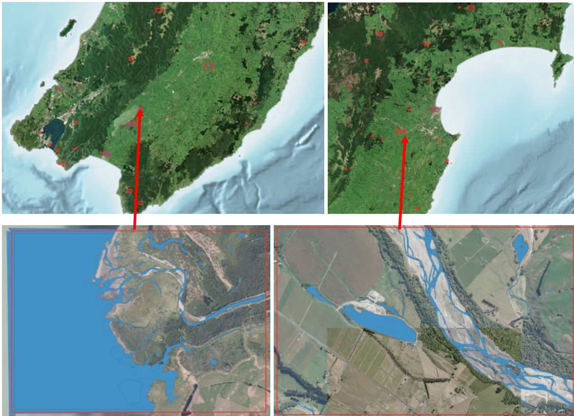
Figure 4. Manual labels for the deep learning water detection model. Training areas (red boxes) and water body polygons (blue-filled polygons) were created in Greater Wellington and Hawke’s Bay.
