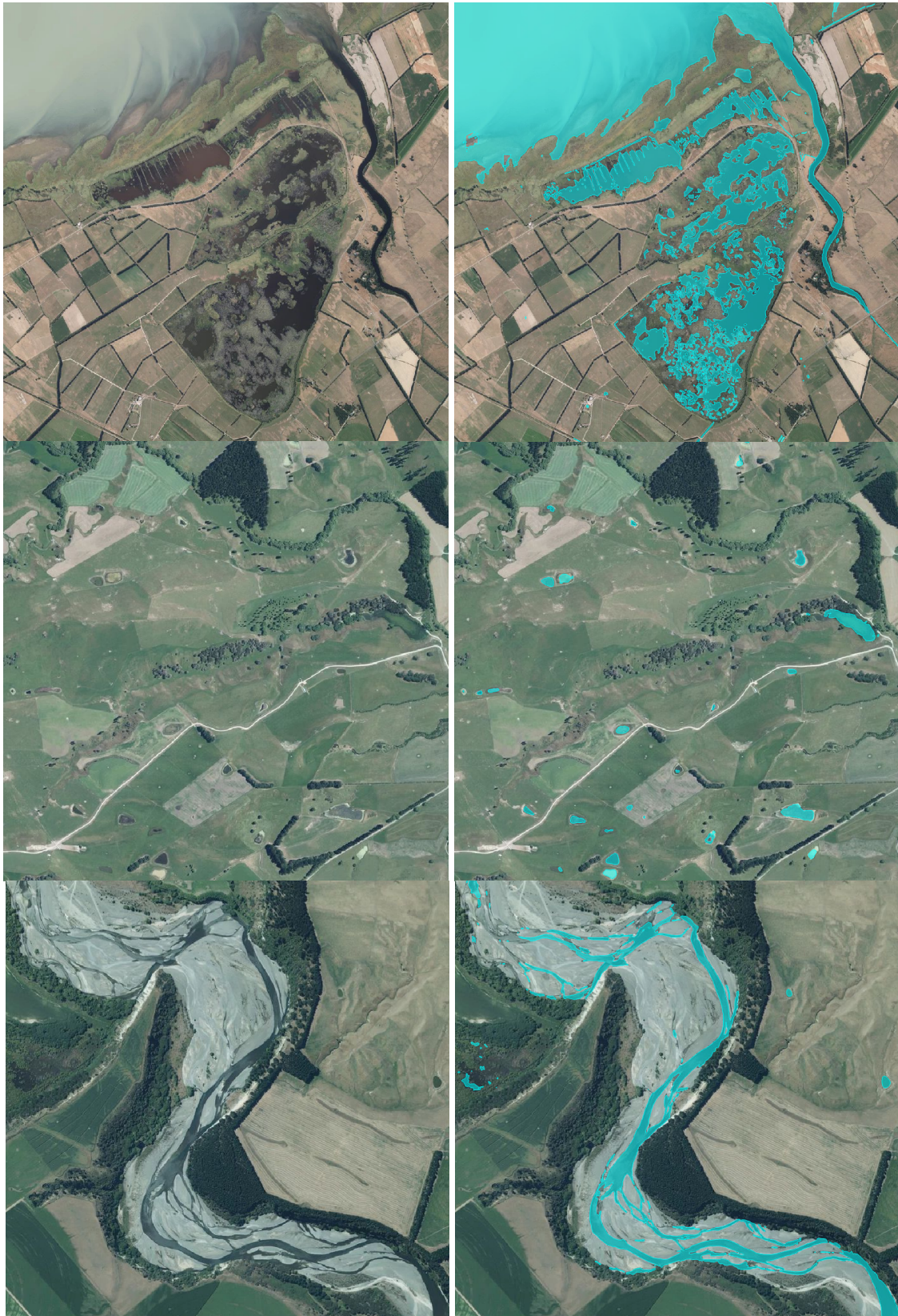
Figure 18. Examples of the deep learning-based water mask for Greater Wellington and Hawke's Bay regions showcasing the spatial detail. Top panels depict the Wairio wetland in Wairarapa, middle panels show kettle holes and small ponds (locality), and bottom panels show complex river systems that are part of the Ngaruroro River in central Hawke's Bay.
