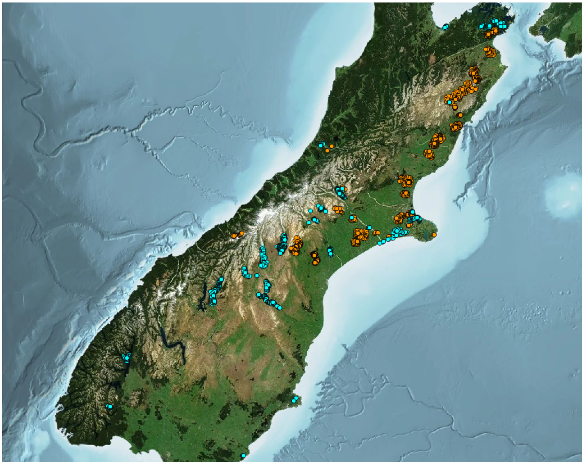
Figure 3. Pseudo ground-truth water (blue) and land (orange) point data manually created in a GIS software.
